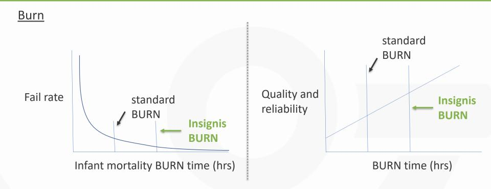
The standard BURN process targets a FIT (Failure In Time) rate for a population of parts. The standard product runs BURN to just meet that FIT target. The Insignis quality material runs an extended BURN time to further improve the population to give an even better FIT rate. Longer BURN times translate into a better quality and reliability experience for Insignis customers.
