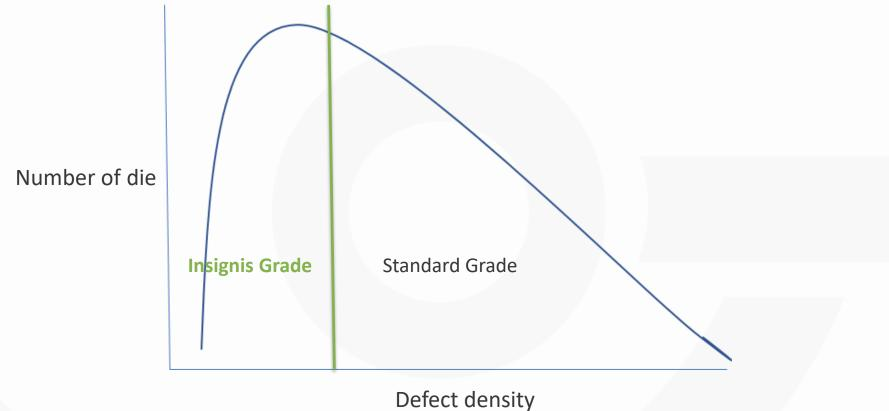
This graph shows the standard distribution of die on a wafer versus the defect density for each die. Every DRAM die requires repair in order to make it a passing die. The number of repairs and the location of the repairs are direct indicators for the defect density for each die.
