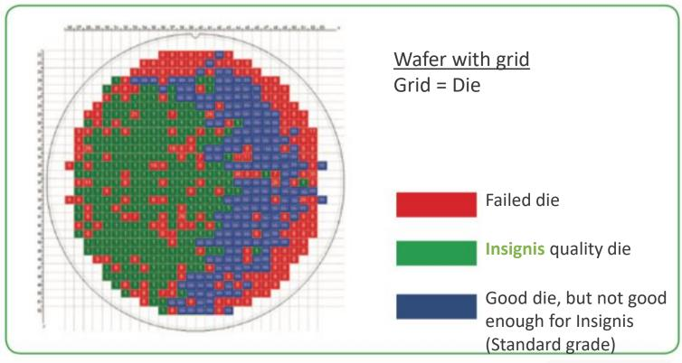
The Insignis test flow selects the die with the lowest defect density to give our customers the best quality and reliability product possible. We have a sophisticated algorithm that screens out die with defects and failure modes that are more likely to fail than the rest of the distribution. The good die on each wafer are further sorted into Insignis grade product and then standard grade product.
