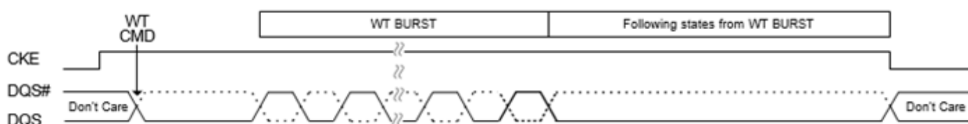
Figure 17. WDQS Control Mode 1 - Read Based Control
