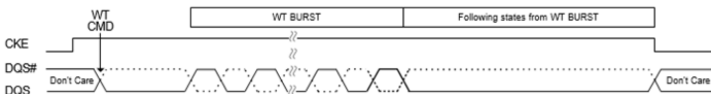
Figure 17. WDQS Control Mode 1 - Read Based Control
