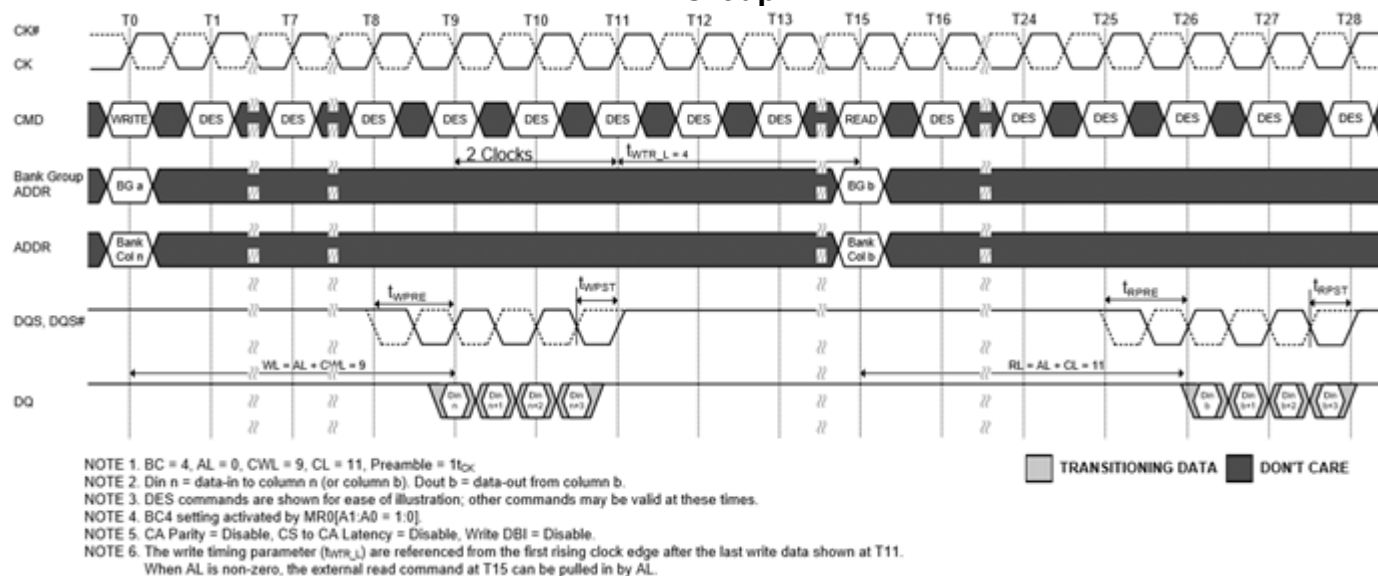
Figure 151. WRITE (BC4)Fixed to READ (BC4)Fixed with 1tCK Preamble in Same Bank Group
