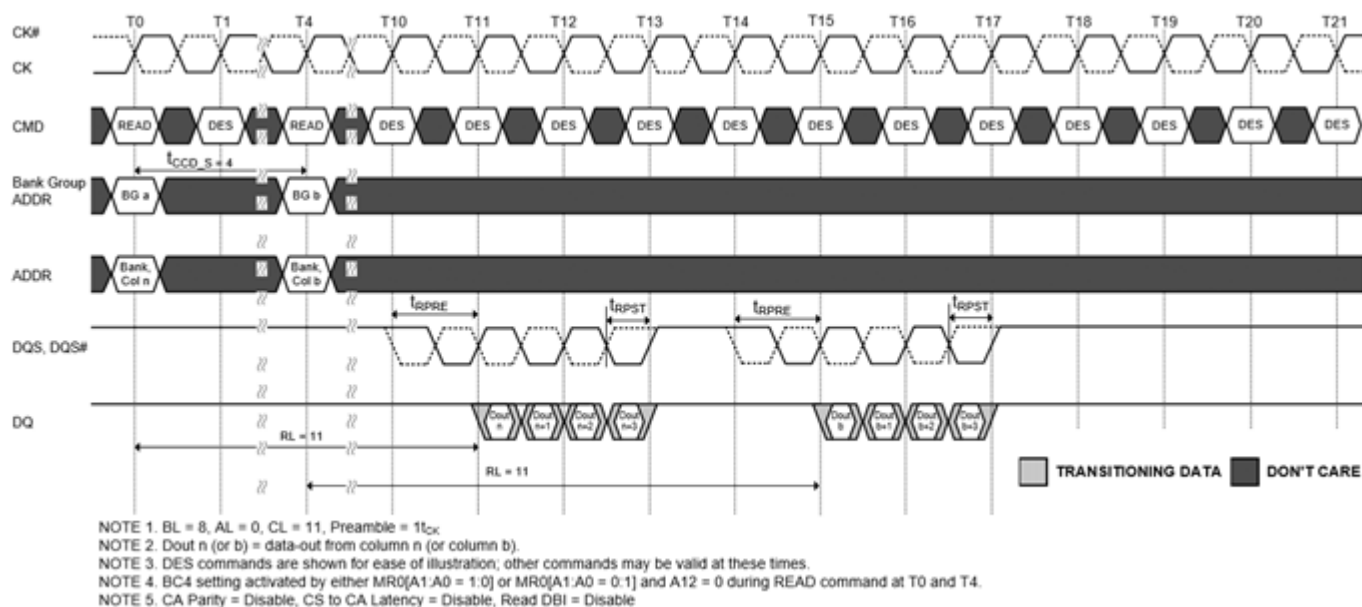
Figure 101. READ (BC4) to READ (BC4) with 1tCK Preamble in Different Bank Group
