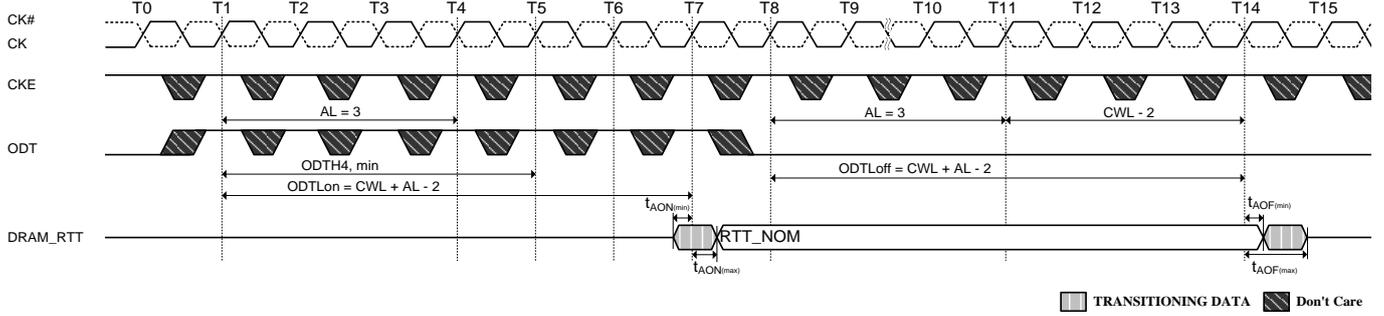
**Figure 68. Synchronous ODT Example with BL = 4, WL = 7**
