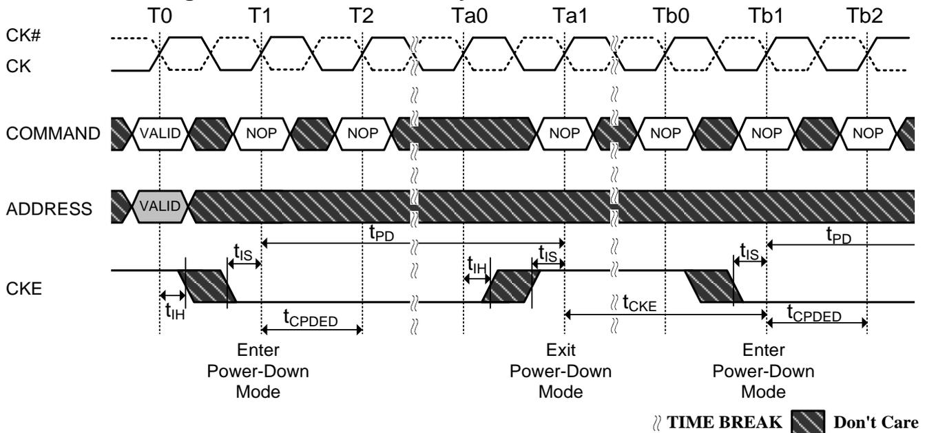
**Figure 80. Power-Down Entry, Exit Clarifications-Case 2**
