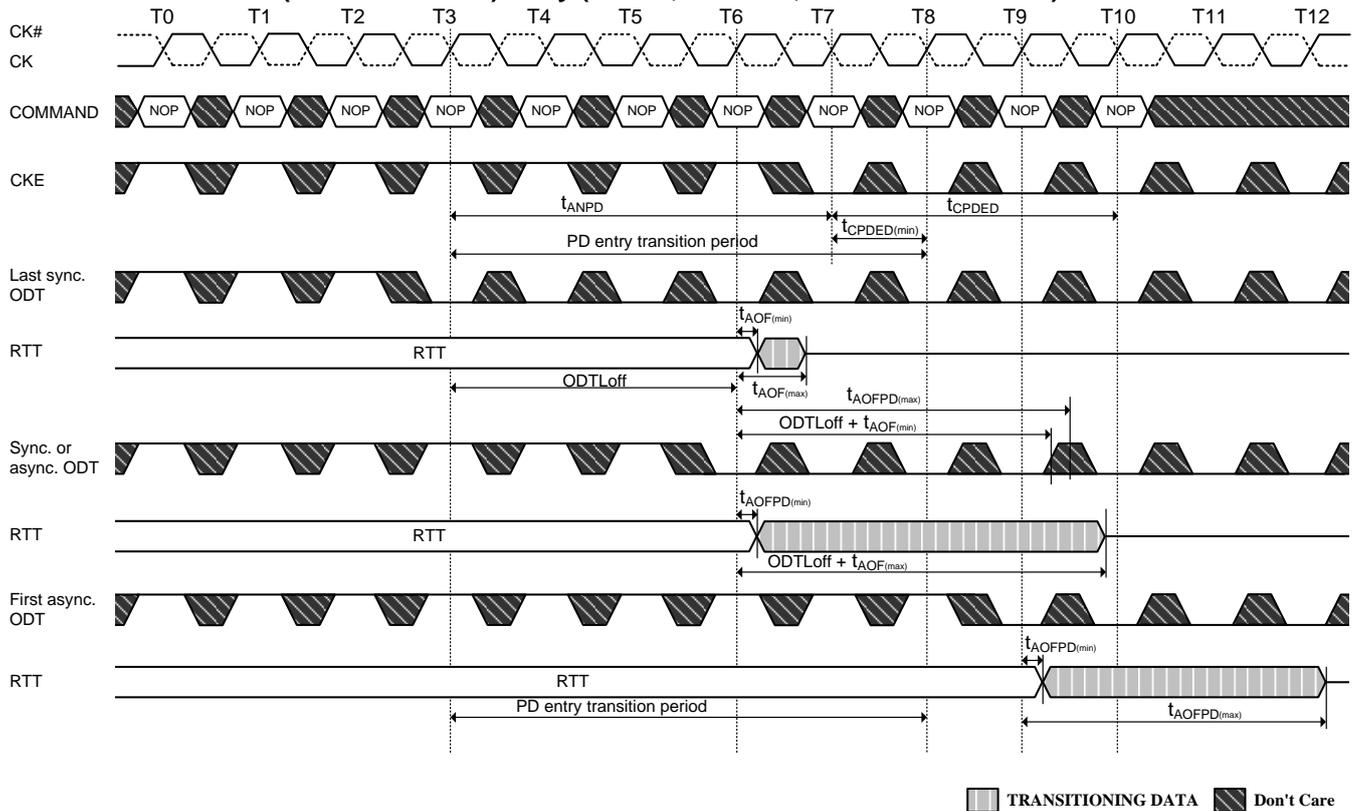
**Figure 76. Synchronous to Asynchronous transition after Refresh Command**
