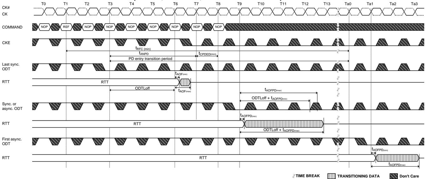
**Figure 77. Asynchronous to Synchronous transition during Precharge Power Down**
