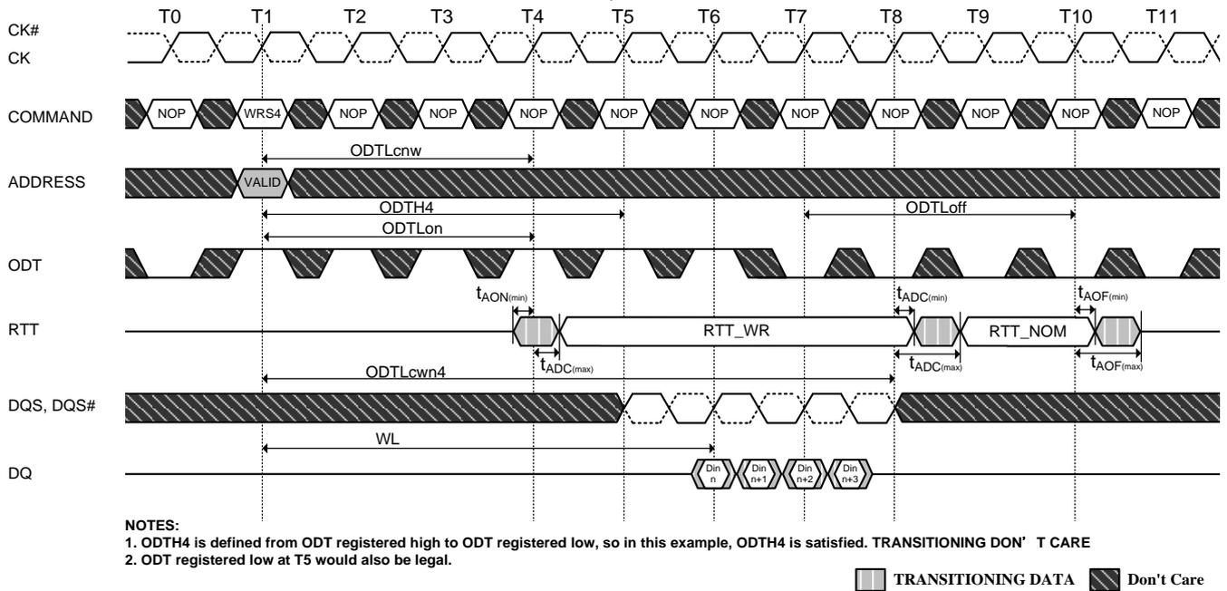
**Figure 73. Dynamic ODT: Behavior with ODT pin being asserted together with Write Command for a duration of 4 clock cycles**
