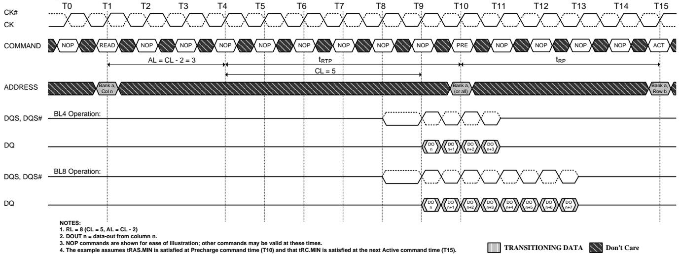
**Figure 43. WRITE Burst Operation WL = 5 (AL = 0, CWL = 5, BL8)**
