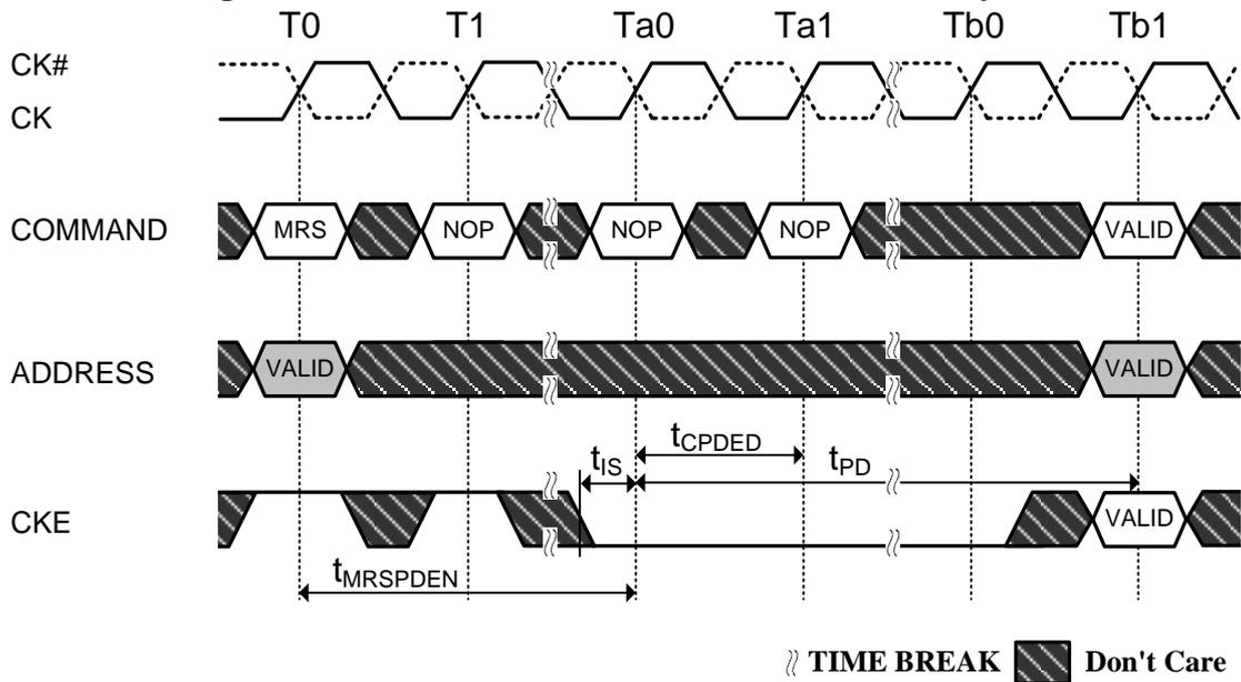
**Figure 67. Synchronous ODT Timing Example**
