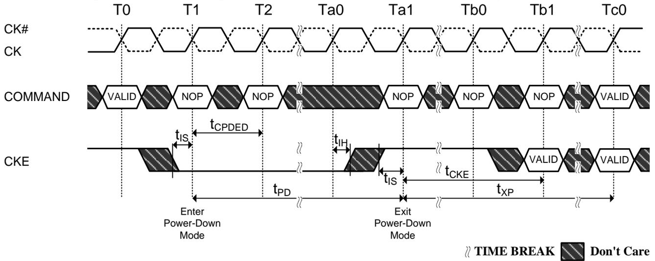
**Figure 62. Precharge Power-Down (Slow Exit Mode) Entry and Exit**
