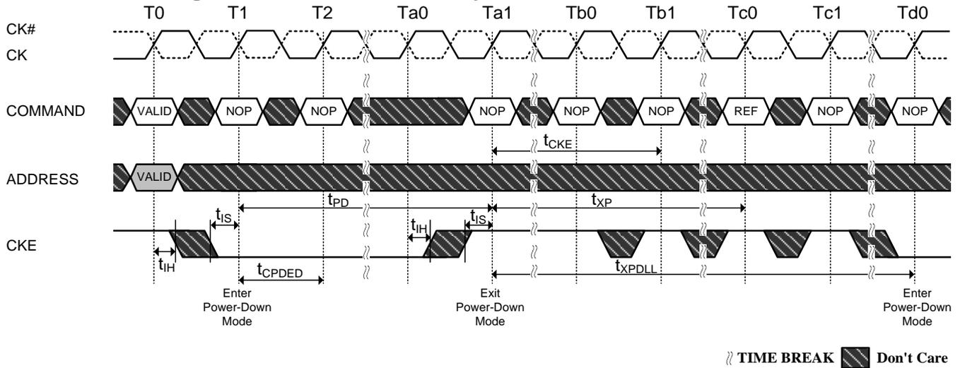
**Figure 81. Power-Down Entry, Exit Clarifications-Case 3**
