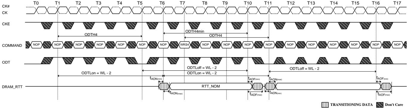
**Figure 69. Dynamic ODT Behavior with ODT being asserted before and after the Write**
