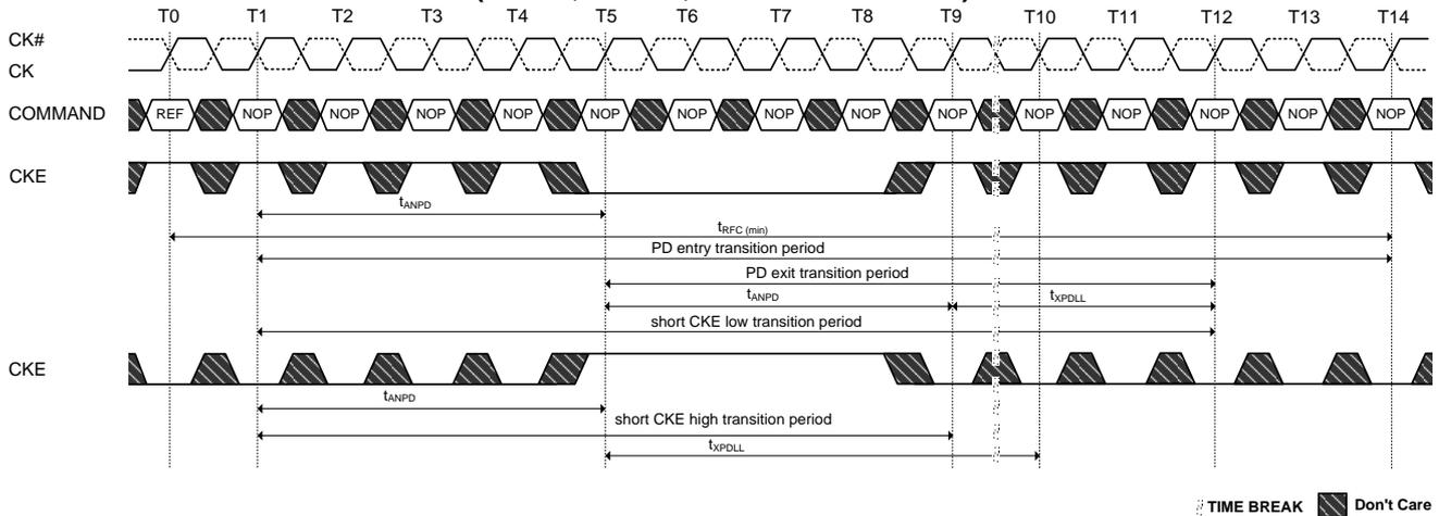
**Figure 79. Power-Down Entry, Exit Clarifications-Case 1**
