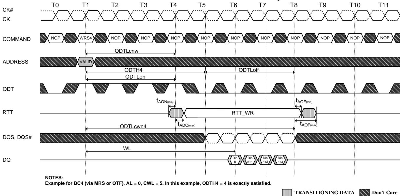
**Figure 74. Asynchronous ODT Timings on DDR3L SDRAM with fast ODT transition**
