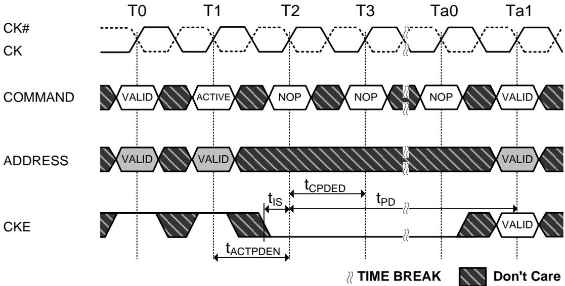
**Figure 65. Precharge, Precharge All Command to Power-Down Entry**
