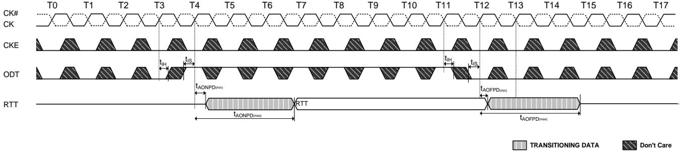
**Figure 75. Synchronous to Asynchronous transition during Precharge Power Down (with DLL frozen) entry (AL = 0; CWL = 5; tANPD = WL - 1 = 4)**
