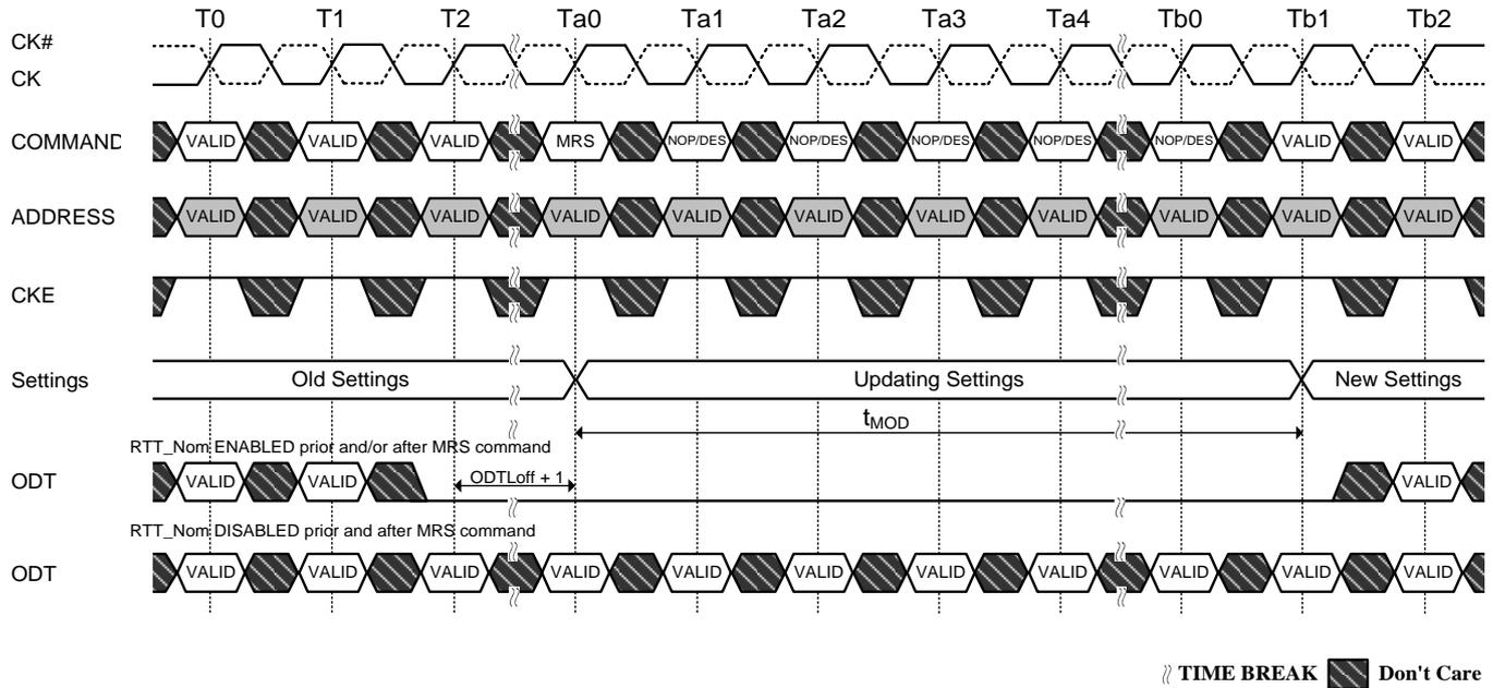
The mode register contents can be changed using the same command and timing requirements during normal operation as long as the DRAM is in idle state, i.e., all banks are in the precharged state with  $t_{RP}$  satisfied, all data bursts are completed and CKE is high prior to writing into the mode register. The mode registers are divided into various fields depending on the functionality and/or modes.
