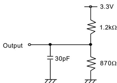
**Figure 18.2 LVTTL A.C. Test Load (B)**
