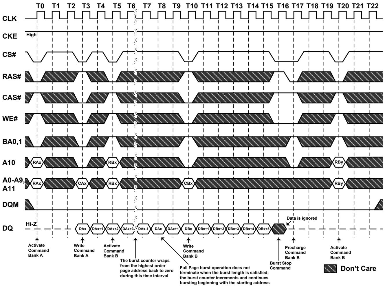
**Figure 38. Byte Read and Write Operation**
