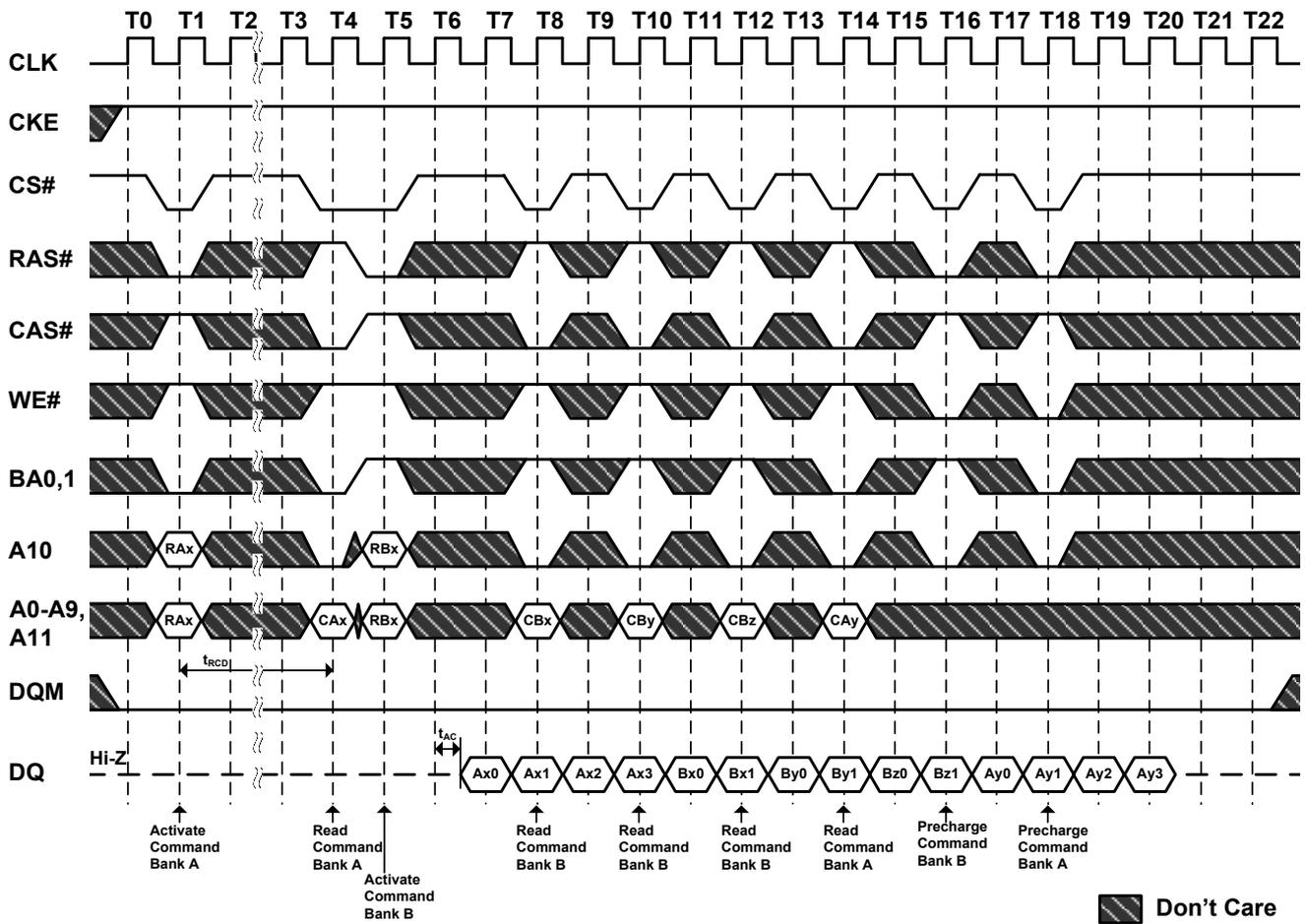
**Figure 33. Interleaved Column Write Cycle**
