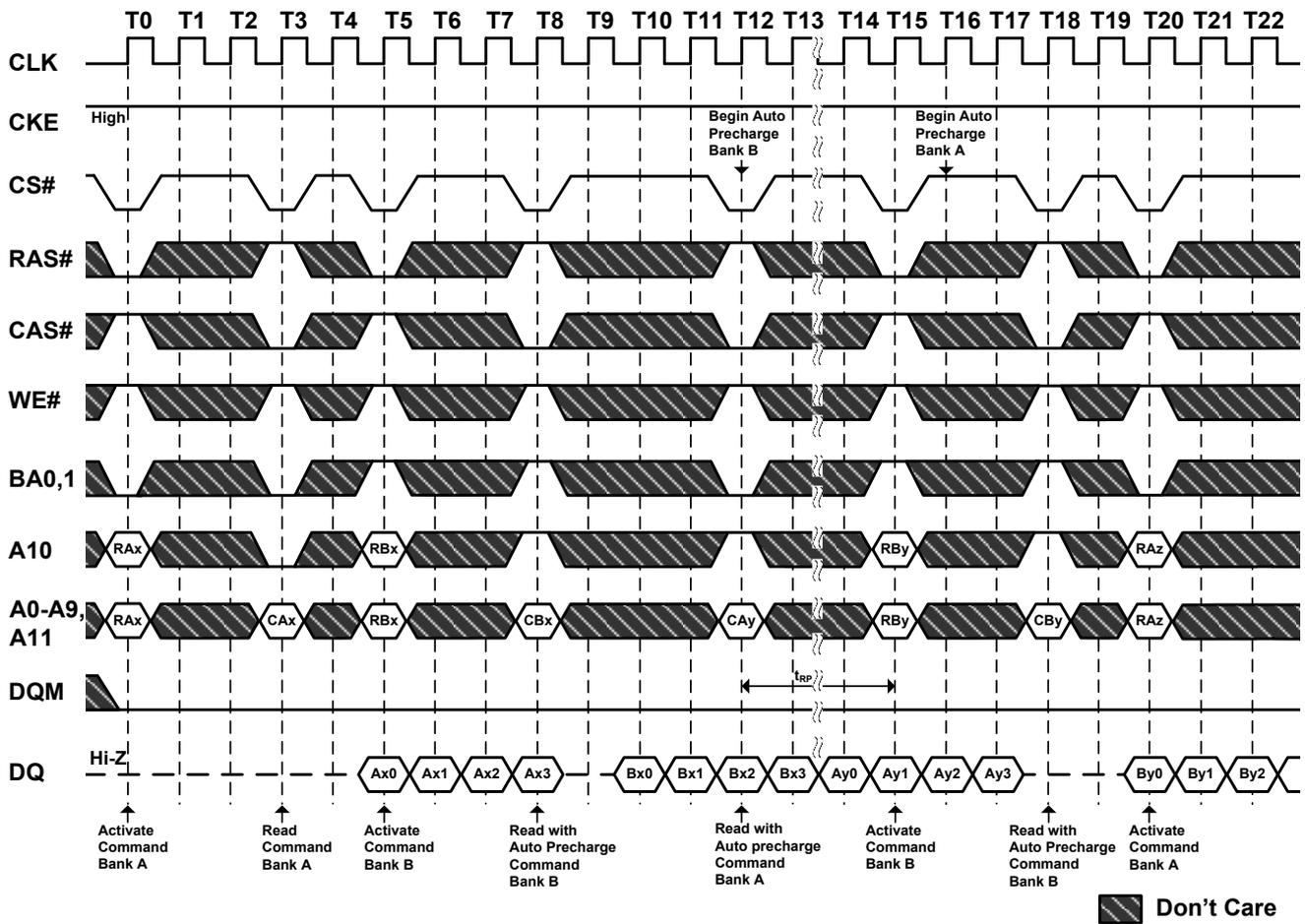
**Figure 34.2. Auto Precharge after Read Burst**
