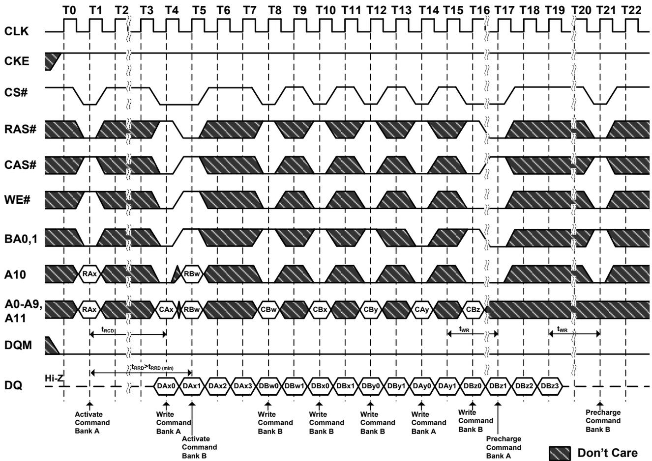
**Figure 34.1. Auto Precharge after Read Burst**
