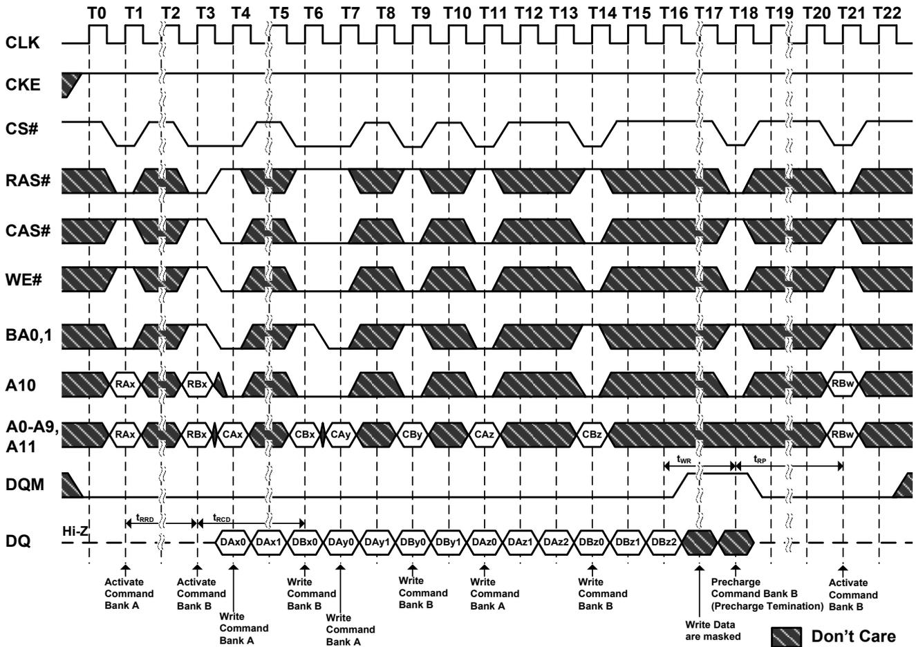
**Figure 42. Precharge Termination of a Burst**
