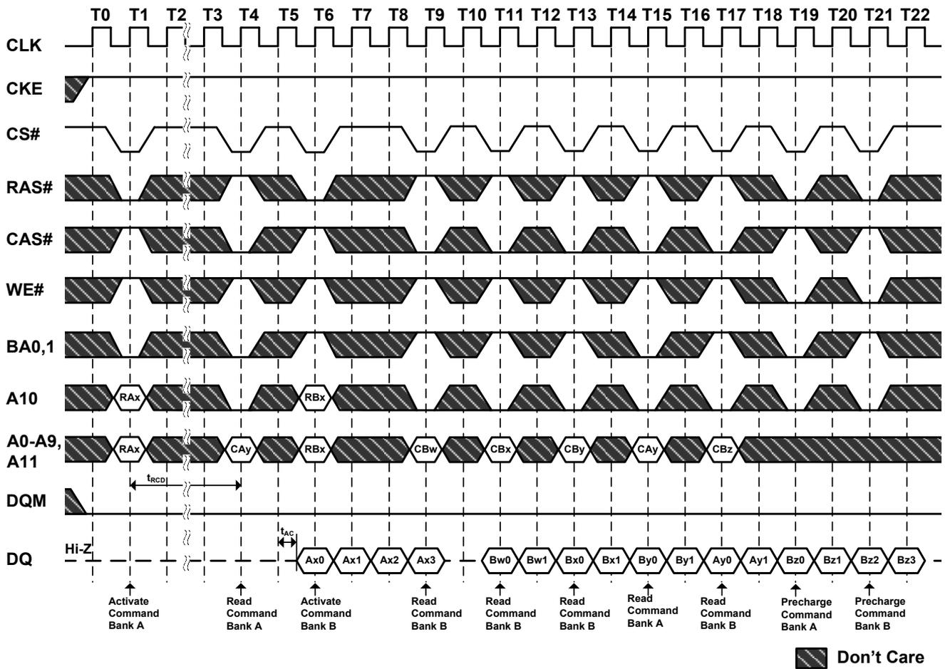
**Figure 32.2. Interleaved Column Read Cycle**
