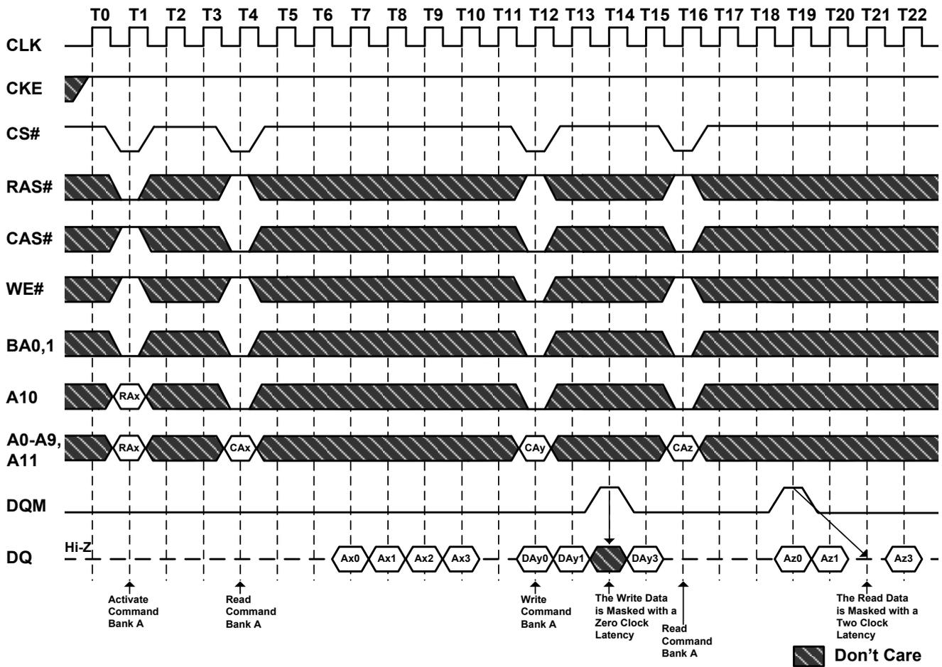
**Figure 32.1. Interleaving Column Read Cycle**
