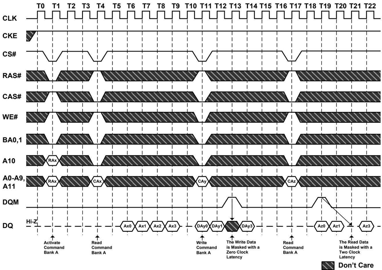
**Figure 31.2. Read and Write Cycle**
