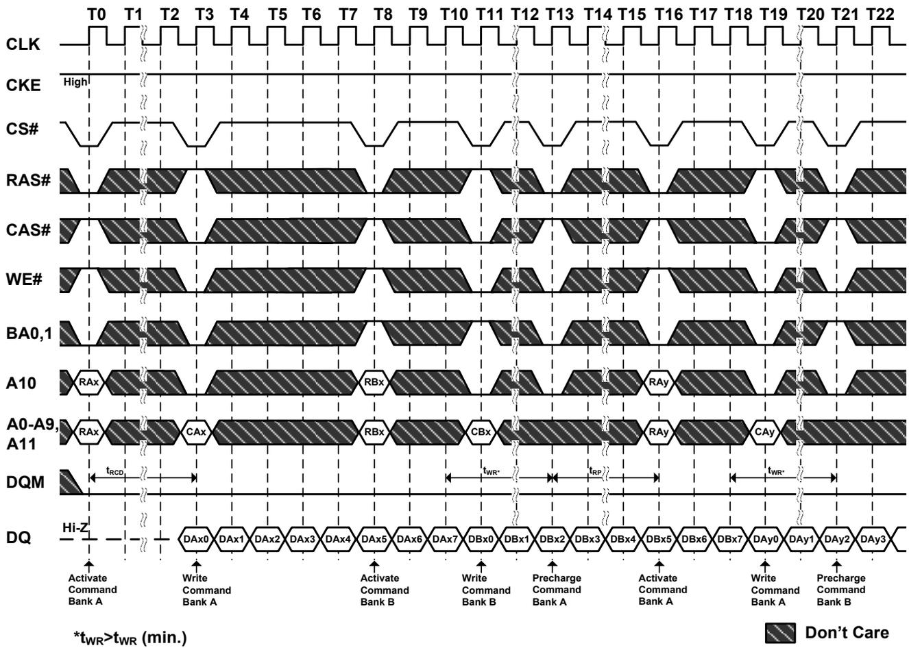
**Figure 31.1. Read and Write Cycle**
