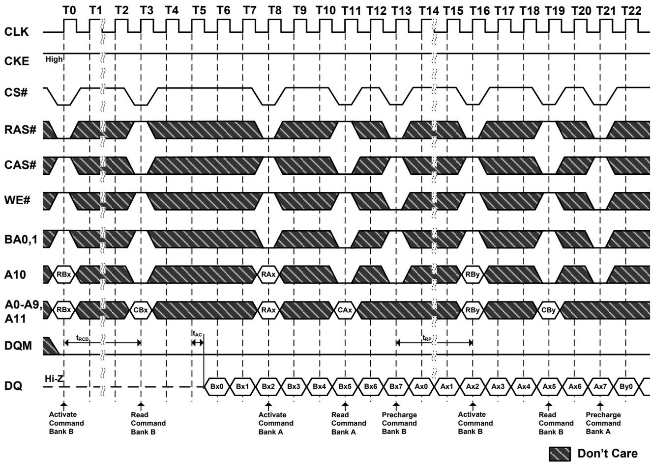
**Figure 30. Random Row Write (Interleaving Banks)**
