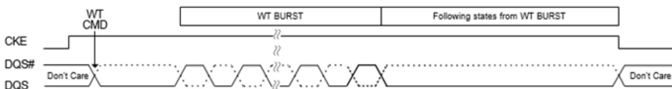
Figure 17. WDQS Control Mode 1 - Read Based Control
