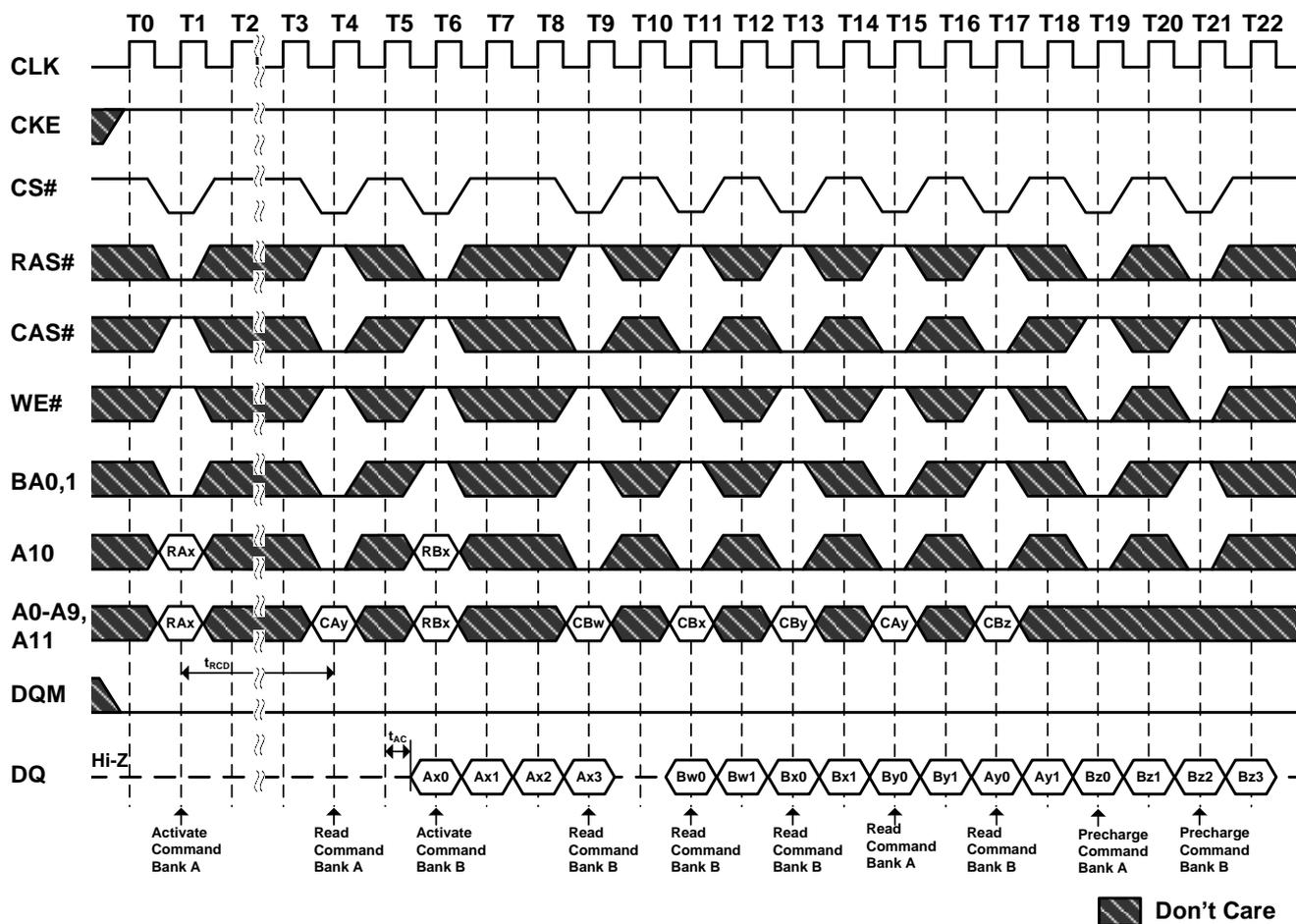
**Figure 32.2. Interleaved Column Read Cycle**
