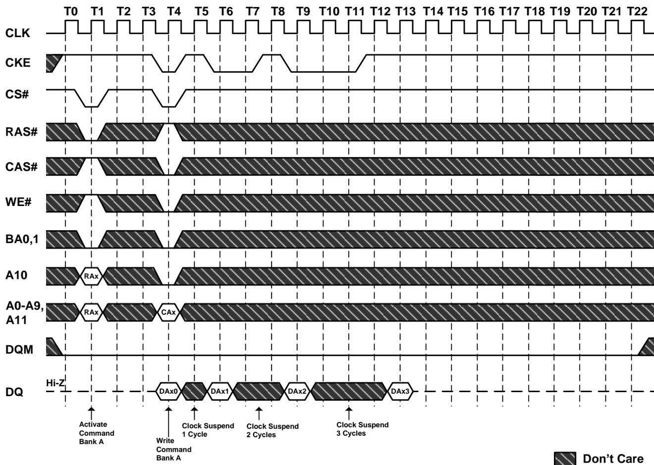
**Figure 26. Power Down Mode and Clock Suspension**
