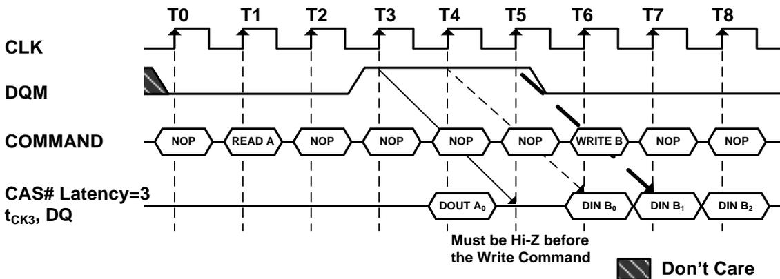
**Figure 8. Read to Write Interval**
