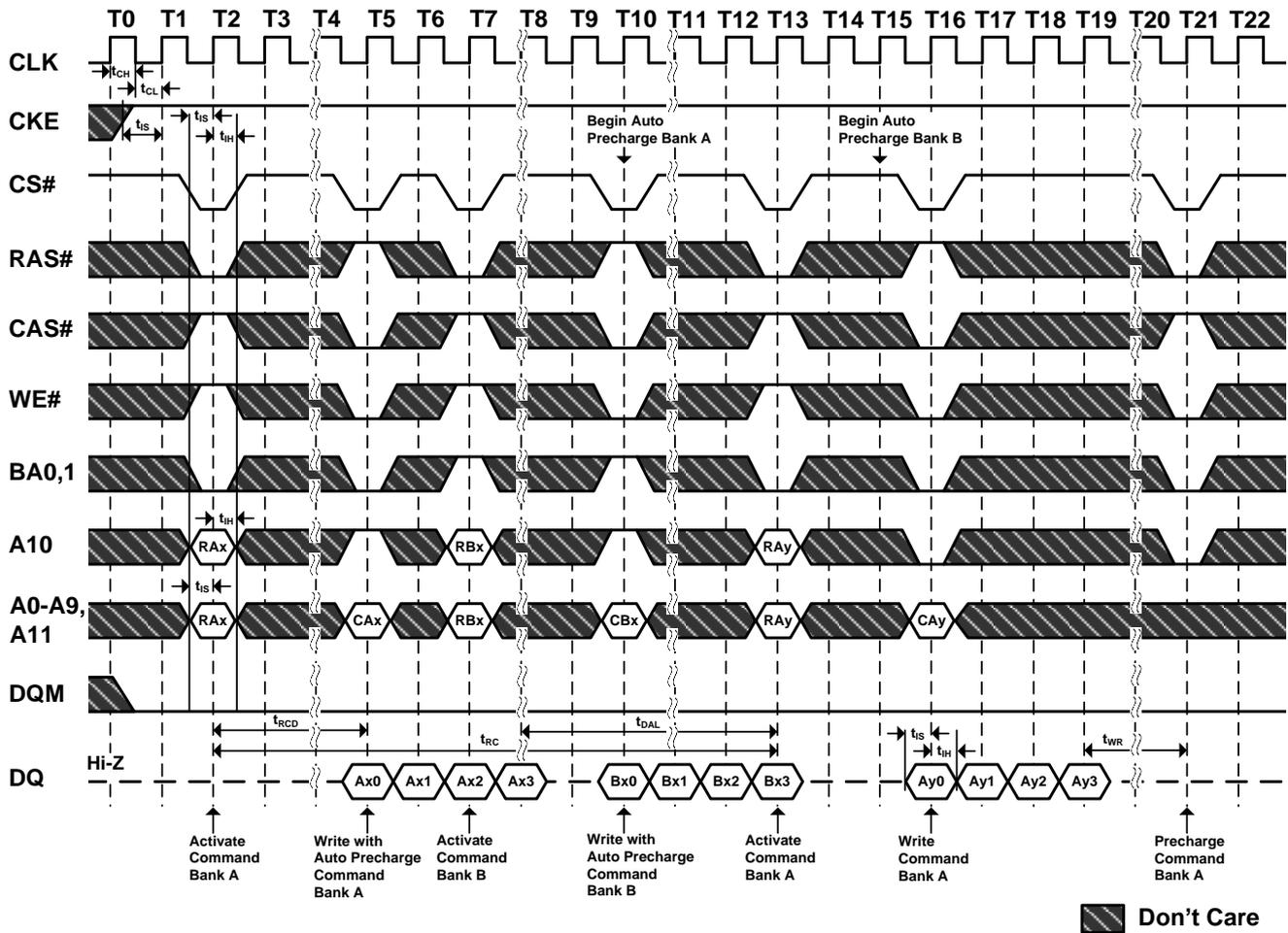
**Figure 20. AC Parameters for Read Timing**
