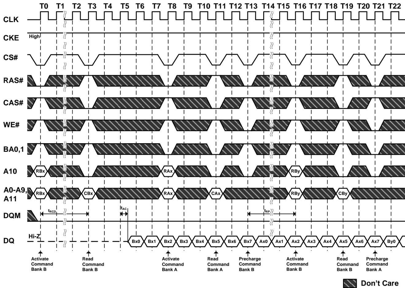
**Figure 30. Random Row Write (Interleaving Banks)**
