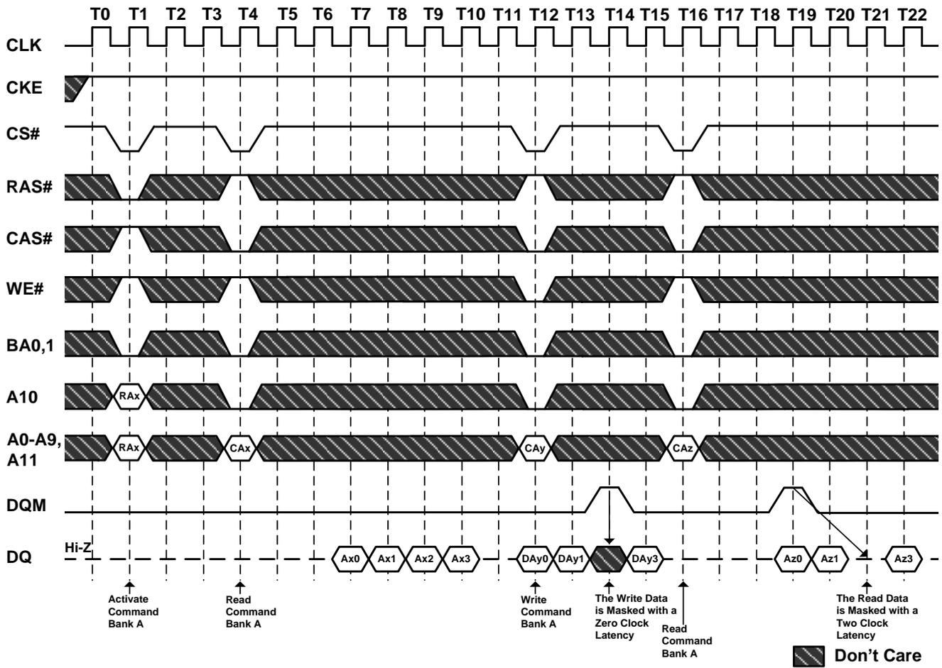
**Figure 32.1. Interleaving Column Read Cycle**
