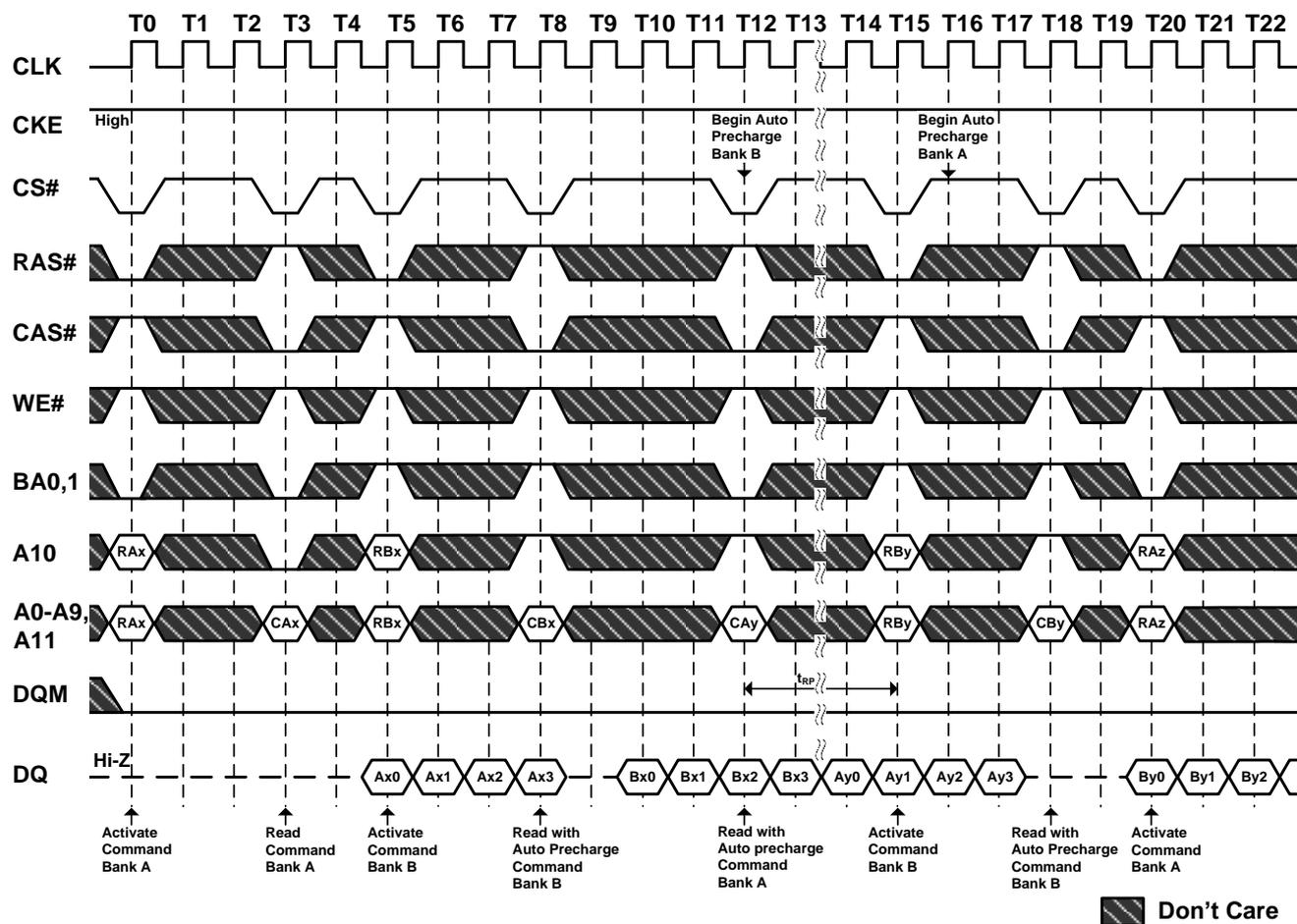
**Figure 34.2. Auto Precharge after Read Burst**
