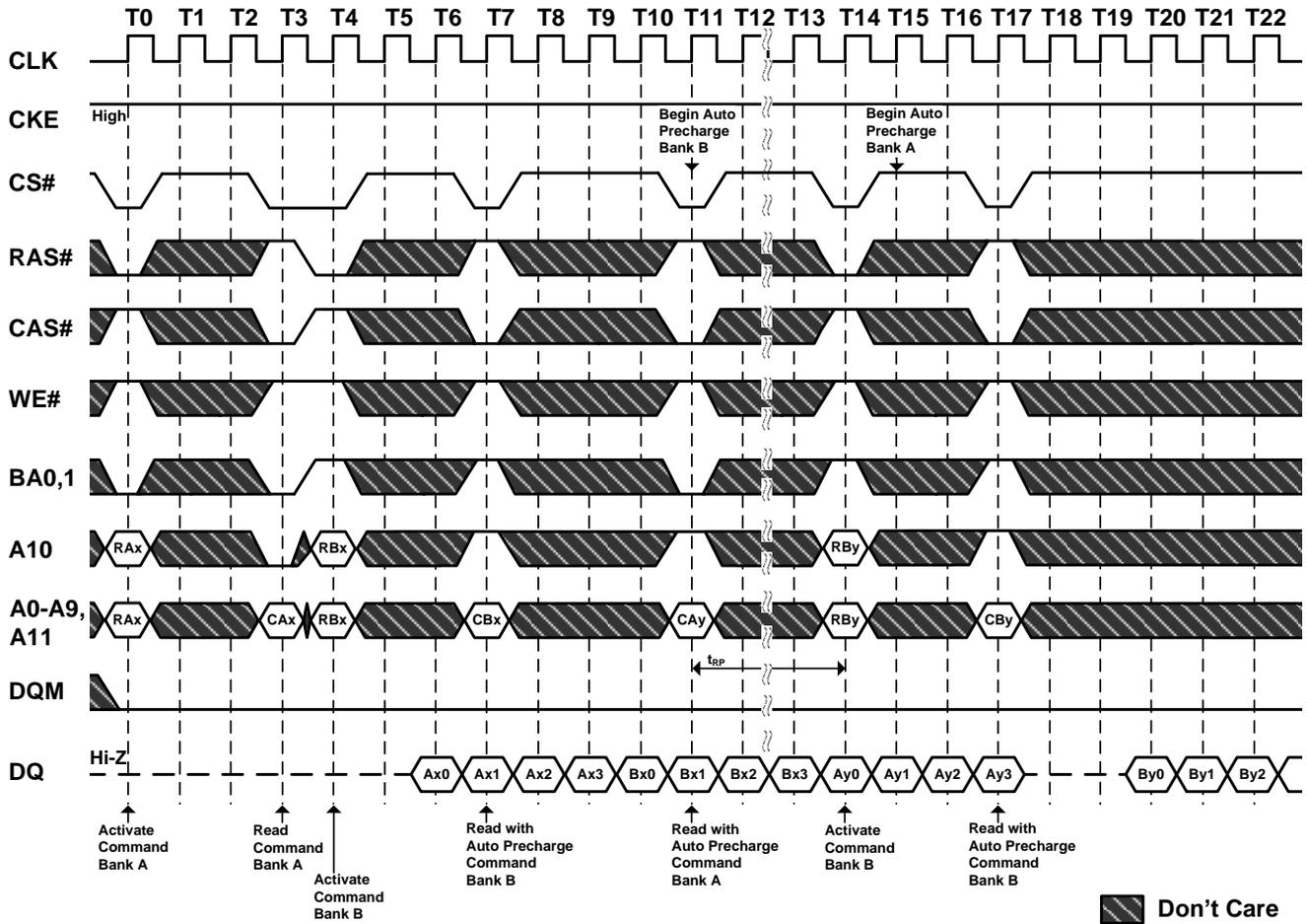
**Figure 35. Auto Precharge after Write Burst
