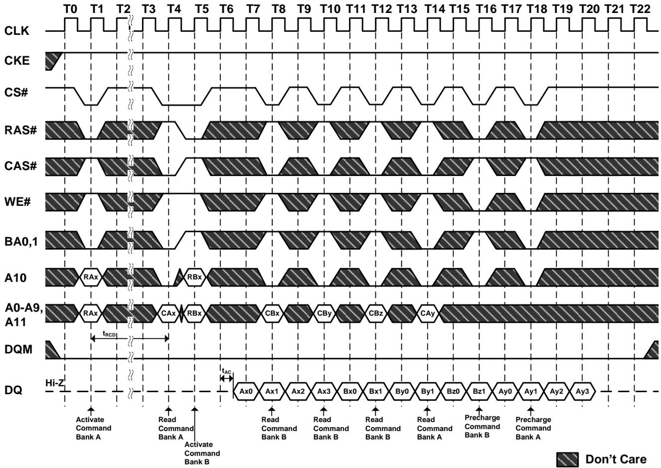
**Figure 33. Interleaved Column Write Cycle
