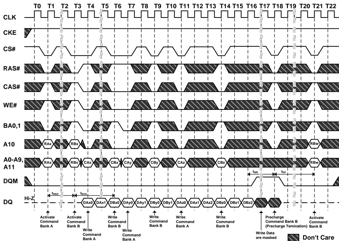
**Figure 42 Precharge Termination of a Burst**
