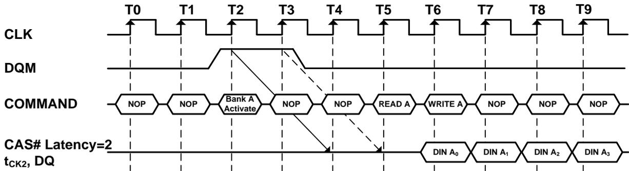
**Figure 7. Read to Write Interval**
