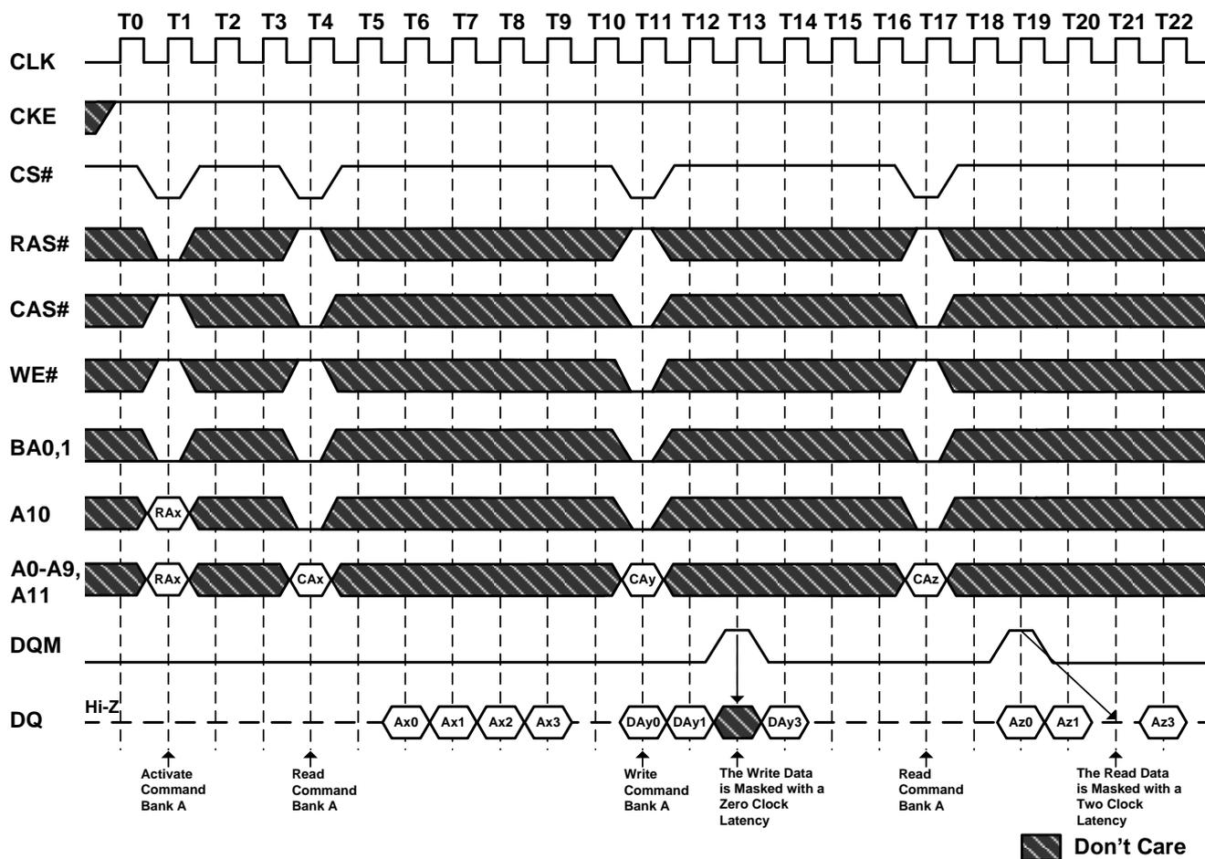
**Figure 31.2. Read and Write Cycle**
