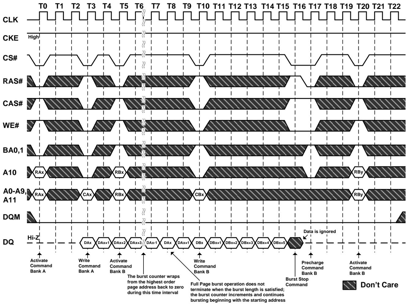
**Figure 38. Byte Read and Write Operation**
