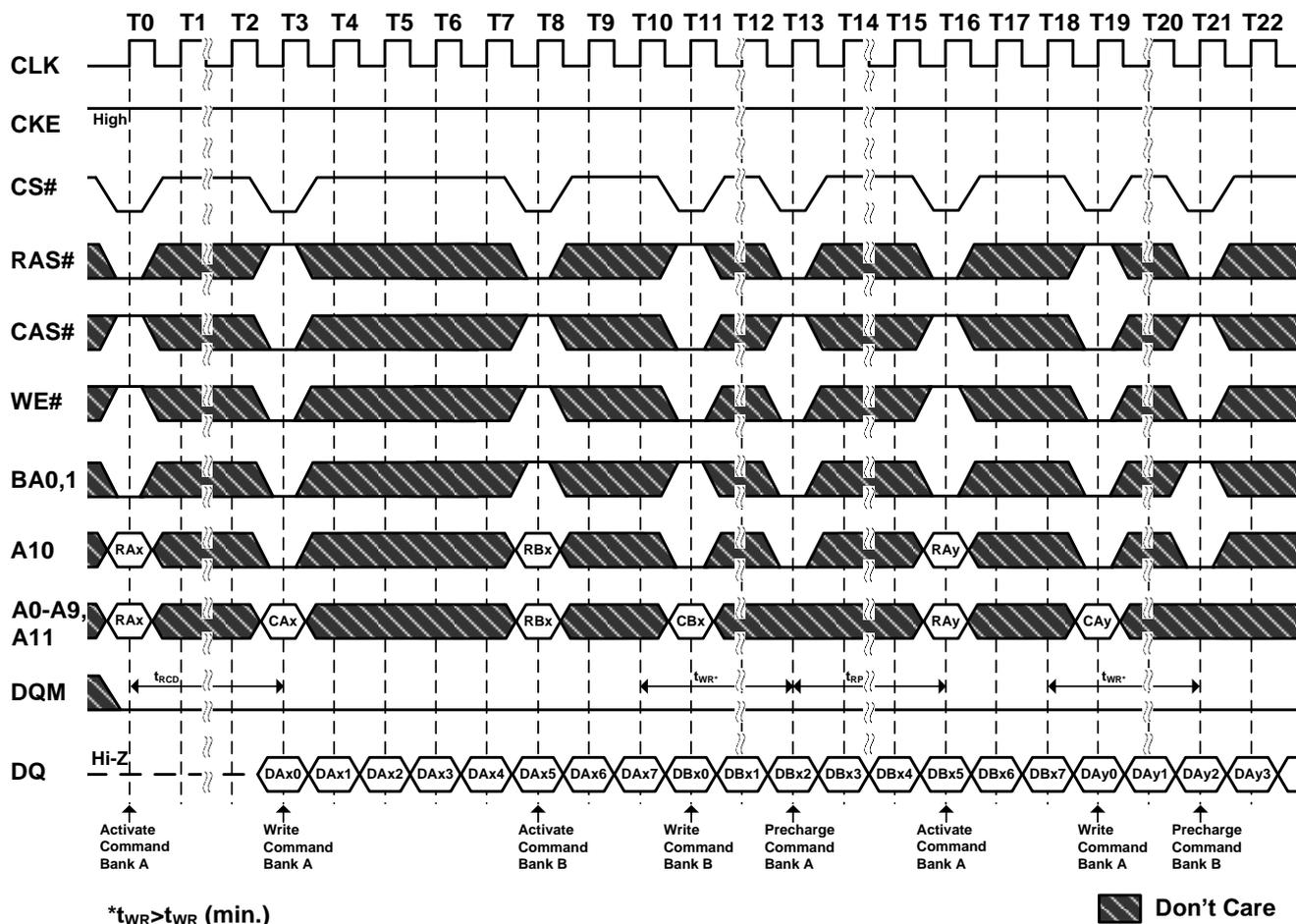
**Figure 31.1. Read and Write Cycle**
